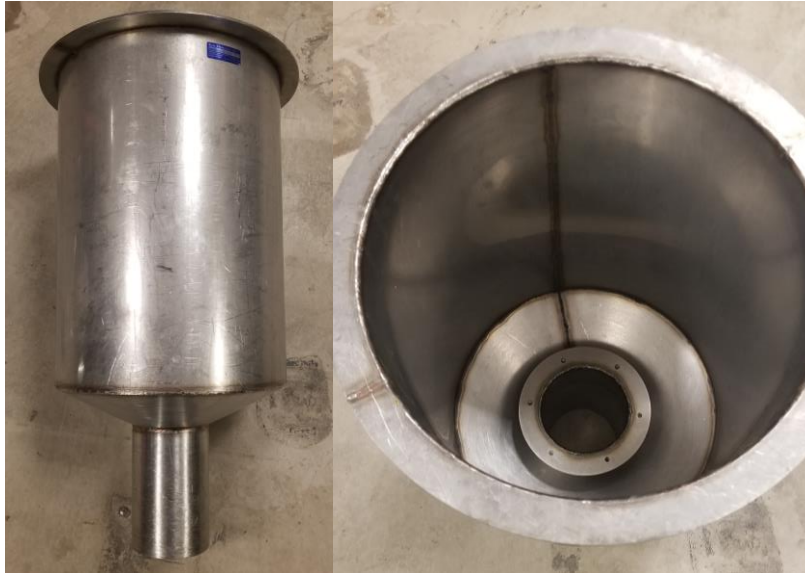
Photo 3-6: Side-view and top-view of the McNeil sampler. Device was driven into the streambed up to the collar and substrate material was removed for analyses from the interior area of the narrow portion.
