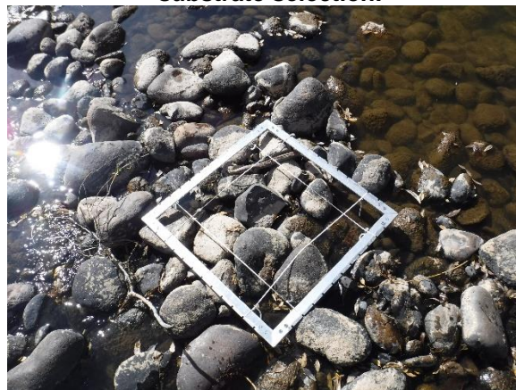
Photo 3-2: Sampling frame with four cross sections for randomized substrate selection.
